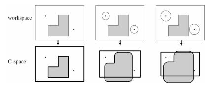
• A consistent reference point must be picked on the robot.
