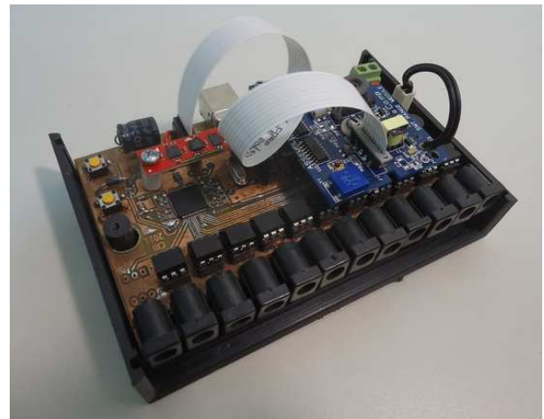
Fig. 7. Developed sensor module for ultrasonic ring and inertial sensor.
