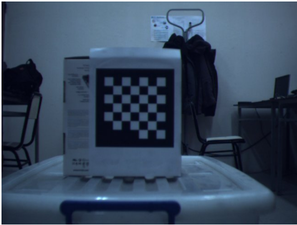
Figure 5.2: distance camera - landmark: 1m
