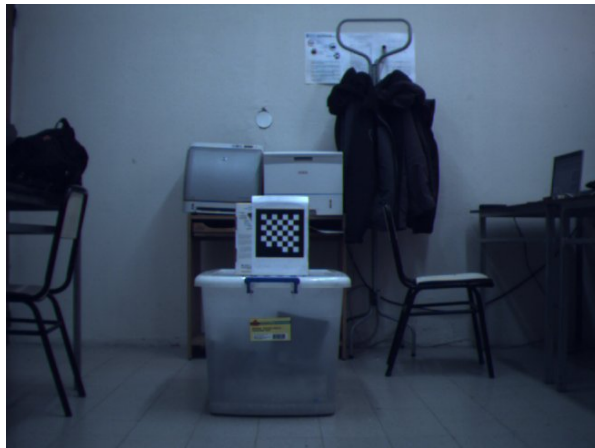
Figure 5.6: distance camera - landmark: 3m
