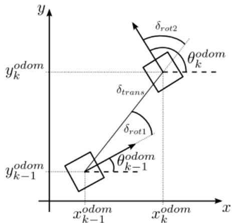
$$\delta_{rot1} = \text{atan2}(y_k^{odom} - y_{k-1}^{odom}, x_k^{odom} - x_{k-1}^{odom}) - \theta_{k-1}^{odom}$$
